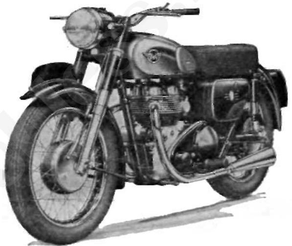
tank decoration. For the first time since rear springing was introduced in 1949 proprietary shock absorbers are used in place of the A.M.C.-manufactured units. In addition to the foregoing changes there are several minor modifications aimed chiefly at cleaning up appearance and eliminating oil leakage.
