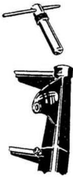
61-3009 Removing Fork Shaft from Front Yoke
